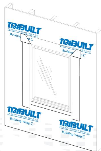
Figure 7: Flashing applied to window header.
