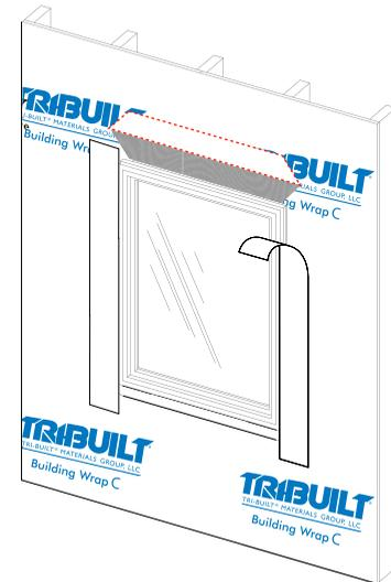
Figure 6: Flashing applied to jambs.
